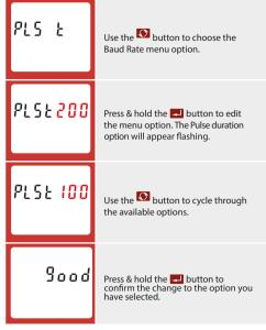
To exit the set-up menu, press & hold 1 until the
