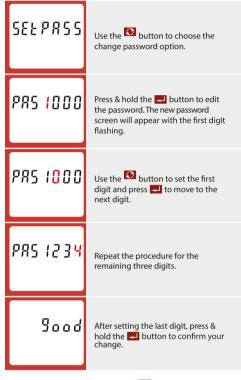
To exit the set-up menu, press & hold 🚺 until the measurement screen is restored
