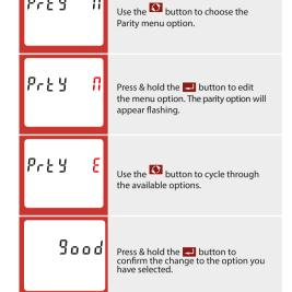
To exit the set-up menu, press & hold 🚺 until the measurement screen is restored.
