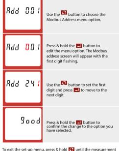
To exit the set-up menu, press & hold 🚺 until the measurement screen is restored.
